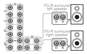
Make sure that the + / – connections are properly inserted (A and B speaker systems are opposite).
